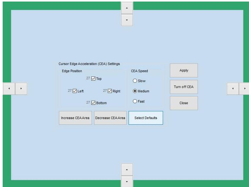
To enable CEA, click on the "Select Default" button and specify the desired parameters. The position of CEA may be manipulated for all edges at once by means of the "Increase/Decrease CEA Area" buttons, or individually by means of the arrows along each edge. Additionally, CEA for particular edges may be disabled by unchecking their respective box.
